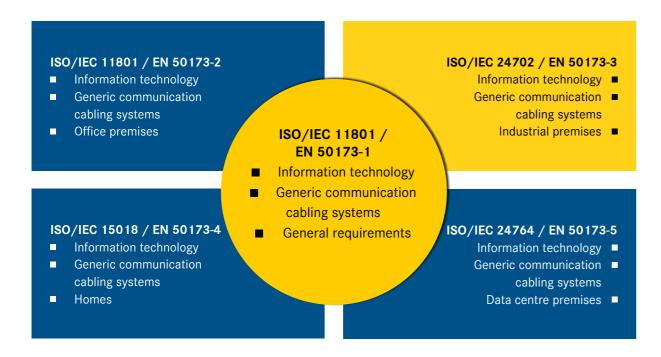
The international cabling standards for structured cabling determine the framework of the HARTING cabling system. The implementation of a standardized cabling system enables networking across high-performance,
